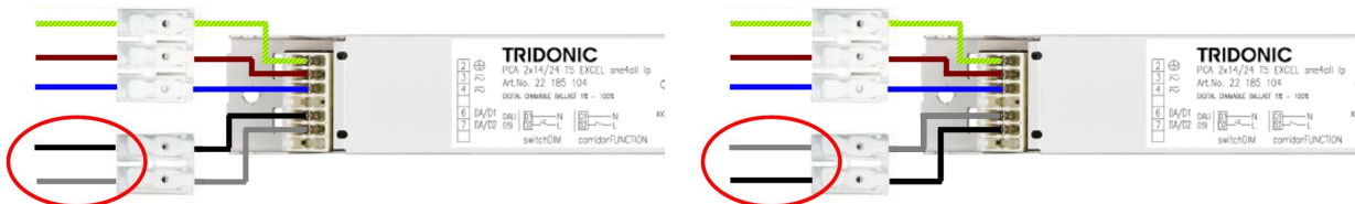
Figure: Different polarity of DALI lines
