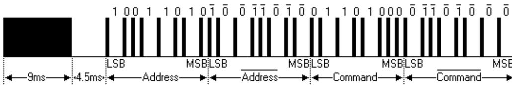
The picture above shows a typical pulse train of the NEC protocol. With this protocol the LSB is transmitted first. In this case Address \$59 and Command \$16 is transmitted. A message is started by a 9ms AGC burst, which was used to set the gain of the earlier IR receivers. This AGC burst is then followed by a 4.5ms space, which is then followed by the Address and
