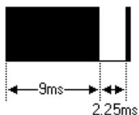
A command is transmitted only once, even when the key on the remote control remains pressed. Every 110ms a repeat code is transmitted for as long as the key remains down. This repeat code is simply a 9ms AGC pulse followed by a 2.25ms space and a 560µs burst.
