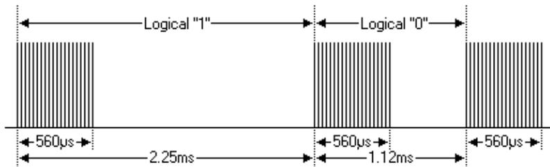
The NEC protocol uses pulse distance encoding of the bits. Each pulse is a 560µs long 38kHz carrier burst (about 21 cycles). A logical "1" takes 2.25ms to transmit, while a logical "0" is only half of that, being 1.125ms. The recommended carrier duty-cycle is 1/4 or 1/3.
