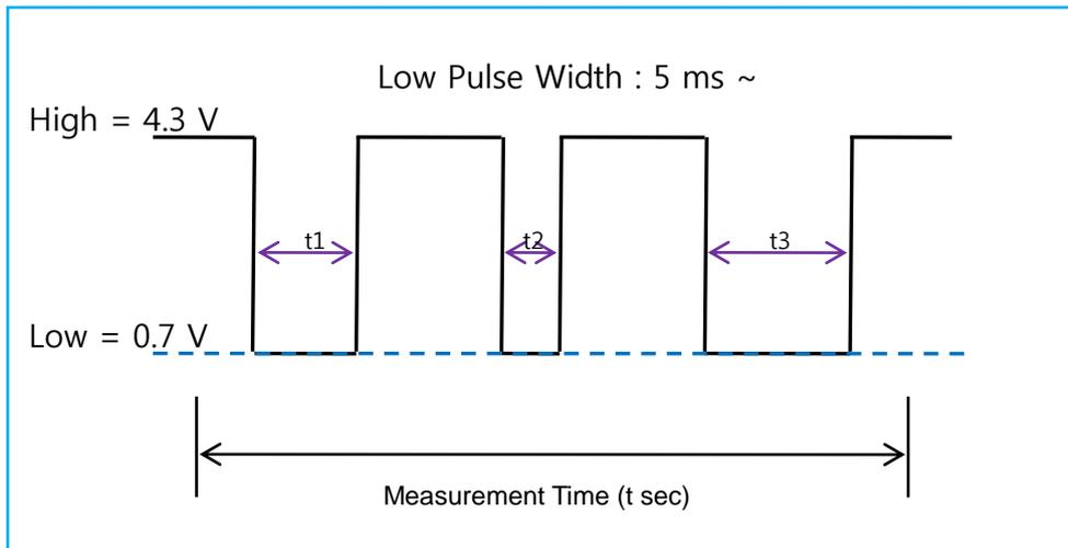
Fig.5 Dust sensor Low Ratio
