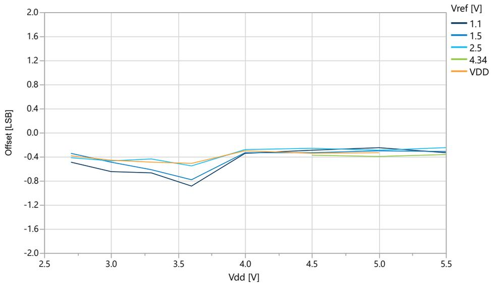
**Figure 36-47. Offset Error vs.  $V_{ref}$  ( $V_{DD}=5.0V$ ,  $f_{ADC}=115$  ksp/s), REFSEL = Internal Reference**
