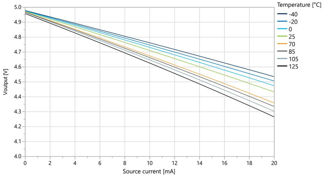
Figure 36-26. I/O Pin Output Voltage vs. Source Current ( $T=25^{\circ}C$ )
