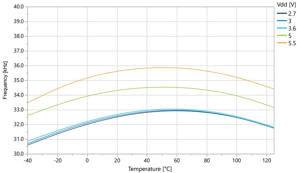
**Figure 36-61. OSCULP32K Internal Oscillator Frequency vs.  $V_{DD}$**
