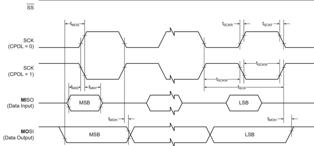
**Figure 35-5. SPI - Timing Requirements in Slave Mode**
