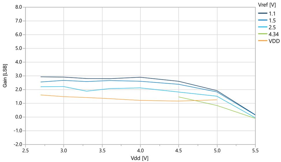
**Figure 36-43. Gain Error vs.  $V_{ref}$  ( $V_{DD}=5.0V$ ,  $f_{ADC}=115$  kps), REFSEL = Internal Reference**
