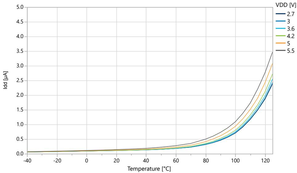
**Figure 36-11. Power Down Mode Supply Current vs.  $V_{DD}$  (All Functions Disabled)**
