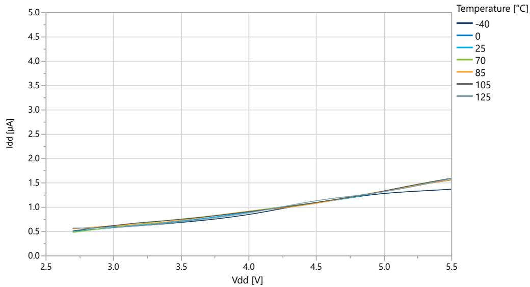
**Figure 36-35. BOD Current vs. V<sub>DD</sub> (Sampled BOD at 1 kHz)**
