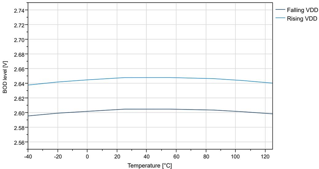
**Figure 36-37. BOD Threshold vs. Temperature (Level 4.3V)**
