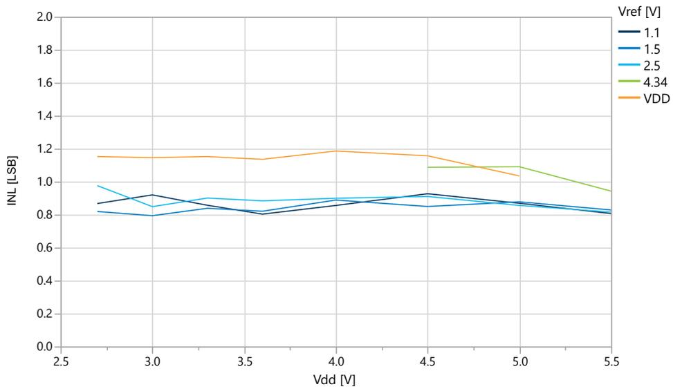
**Figure 36-45. INL vs.  $V_{ref}$  ( $V_{DD}=5.0V$ ,  $f_{ADC}=115$  kps), REFSEL = Internal Reference**
