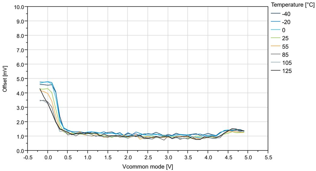
**Figure 36-51. Offset vs.  $V_{CM}$  - 10 mV to 50 mV ( $V_{DD}=5V$ ,  $T=25^{\circ}C$ )**
