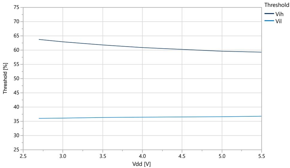
**Figure 36-19. I/O Pin Input Threshold Voltage vs.  $V_{DD}$  ( $V_{IH}$ )**
