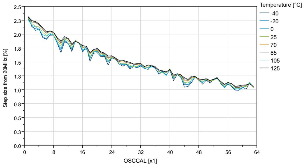
**Figure 36-57. OSC20M Internal Oscillator: Frequency vs. Calibration Value ( $V_{DD}=3V$ )**
