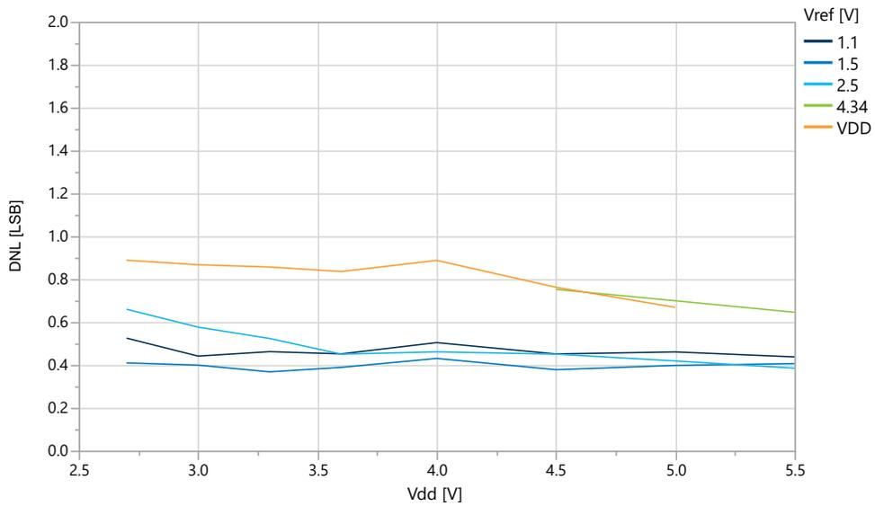
**Figure 36-41. DNL vs.  $V_{ref}$  ( $V_{DD}=5.0V$ ,  $f_{ADC}=115$  ksp/s), REFSEL = Internal Reference**
