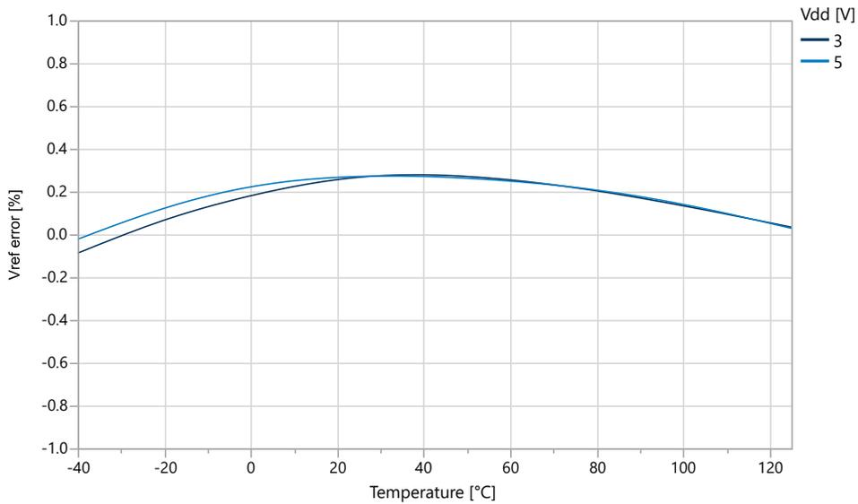
Figure 36-31. Internal 2.5V Reference vs. Temperature
