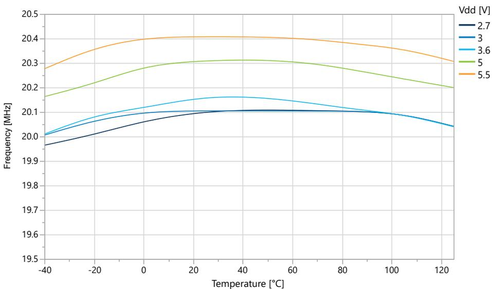
**Figure 36-59. OSC20M Internal Oscillator: Frequency vs. V<sub>DD</sub>**
