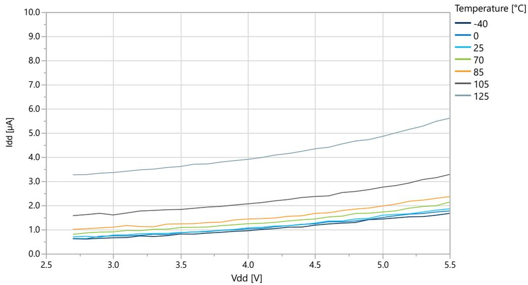
**Figure 36-15. Standby Mode Supply Current vs. V<sub>DD</sub> (Sampled BOD Running at 1 kHz)**
