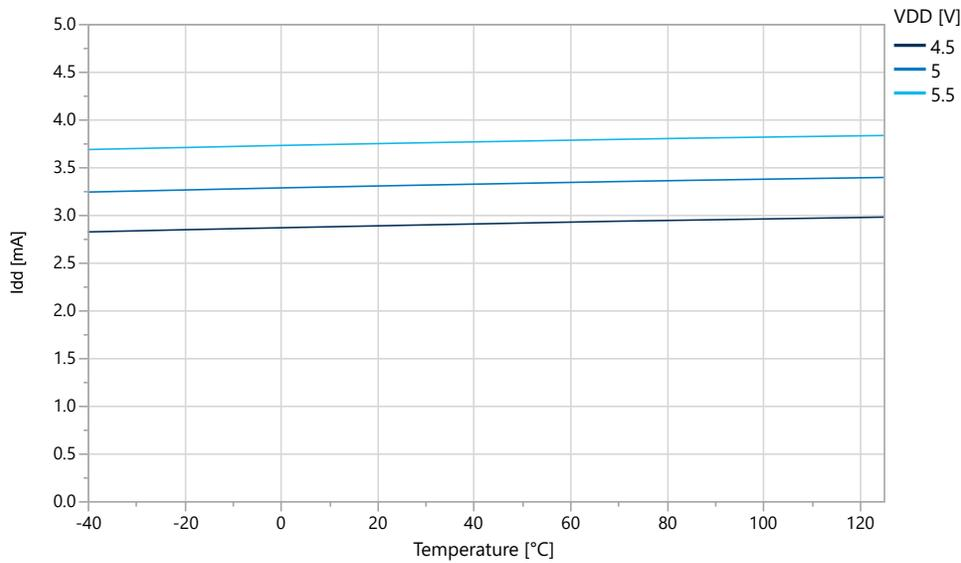
**Figure 36-9. Idle Supply Current vs.  $V_{DD}$  (f=32 KHz OSCULP32K)**
