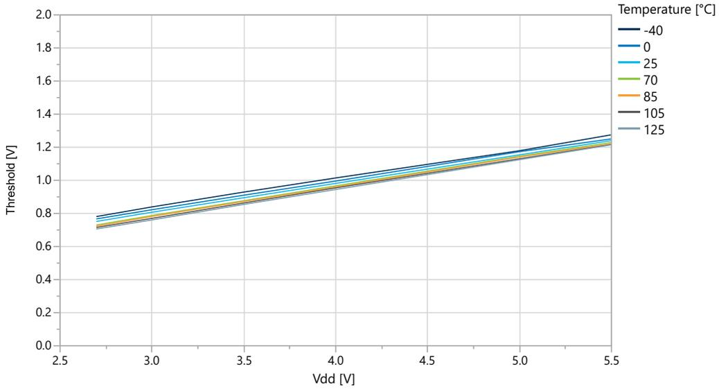
**Figure 36-18. I/O Pin Input Threshold Voltage vs.  $V_{DD}$  (T=25°C)**
