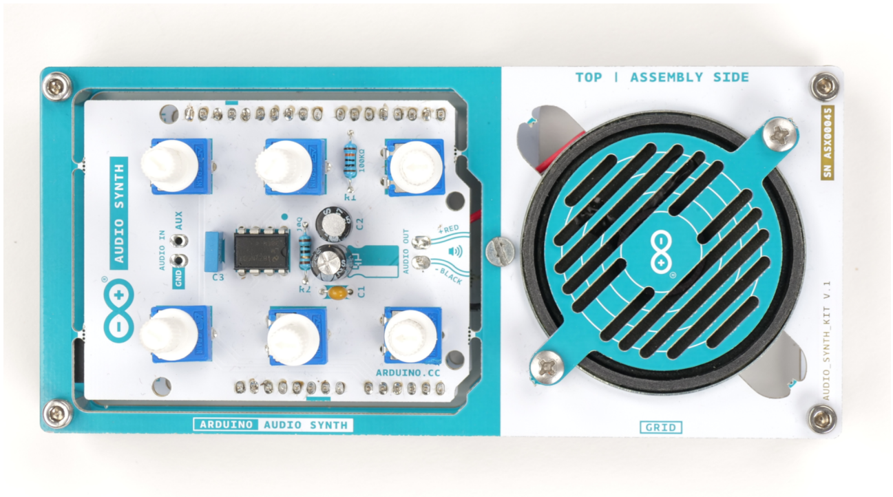
Audio Synth Shield assembled
